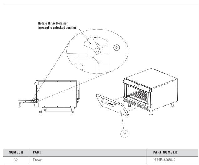
FIGURE 51: Removing the Oven Door
